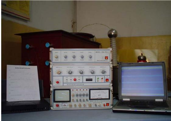
The location detector of PD is developed by Samgor up to minute. It can test and locate discharge of the electrical equipment. It adopts the sonic-electricity and three-dimensional space transducer, which has the patent technology. It can accurately determine space location of the discharge of testing without connecting. It is widely used to locate and detect the partial discharge for dry-transformer, switch, circuit breaker, cable terminal and other the various electrical equipments.
