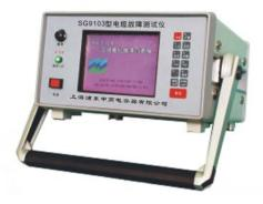
comparison simultaneous display, and it is movable; automatically fault distance calculation, doesn't have artificial conversion; can store test waveforms. The device has printing port, can print all text, graphics and waveform.
