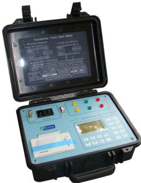
SG7001 is an important basic measurement for power transformer diagnosis. It helps to detect faulty transformer windings as well as defective tap changer positions. This advanced instrument automatically recognizes winding connections and vector group numbers of transformer windings. Just connect the measuring cables and press the start button and get the test results.
