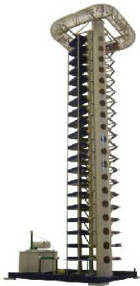
4000kV/400kJ H Structure
