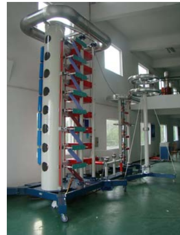
800kV/40kJ L Structure
